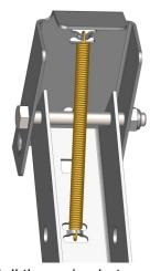
Install the spring between the front edge of the cover and the back profile.
