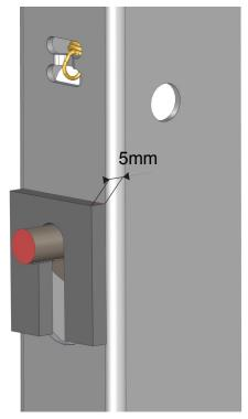
To ensure that the lock cover has play, a space of at least 15mm between the wall and the ladder is required. If the wall is uneven use shims washers as inserts.
