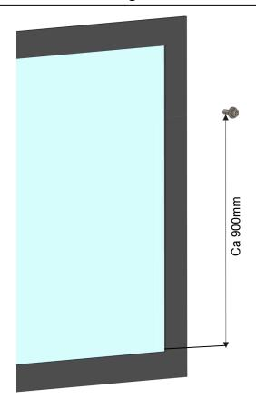
Fasten the first mounting point to the wall. Use suitable bolting material. See MA1001 for screw loads.
