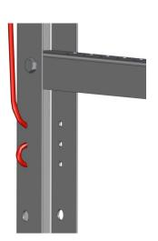
Adjust the length and fasten the wire further down to the side of the ladder. NOTE! Function test.
