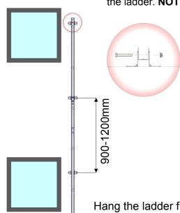
Hang the ladder from the top pair of brackets using M10x60 bolt + nut and solder into place. Then mount the remaining bracket pairs
