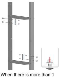
When there is more than 1 module, the ladders are joined together by 2 profiles and 4 M8 coach bolts + nuts.
