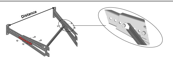
Mount the top brackets first. Determine the suitable length of the bracket and measure the **distance** between the fixing holes. The diagonal brace is mounted in the same hole as the ladder side and to the next innermost hole on the bracket using 4 M10x20 + nuts. For the wall, use max. M12 bolts suitable for wall constructions. *For information about pull out loads see MA1001*
