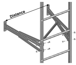
Assemble the other brackets on the ladder using 4 M10x20 bolts + nuts. Max. distance between brackets: **2500 mm.** The diagonal struts are mounted **crosswise**.
