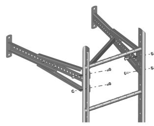
Lift up the ladder and mount in the top brackets.
