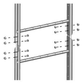
If necessary, the ladders are joined together using the associated joint set and 8 M10x20 + nuts.
