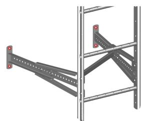
Then bolt the wall brackets on to the façade using suitable bolting material.
