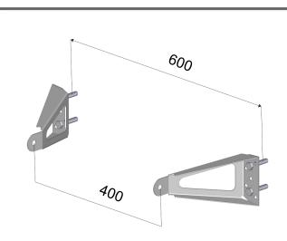
Install the top pair of brackets using suitable bolting material. See MA1001 Loading table for more info.
