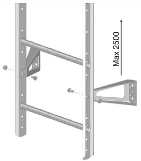
Install the remaining brackets with max. c/c distance of 2500 mm.
