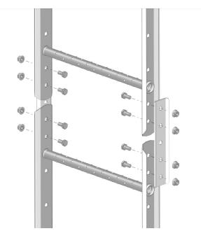
Join the ladders together using joint plate and 4 M10x20 bolts + nuts.
